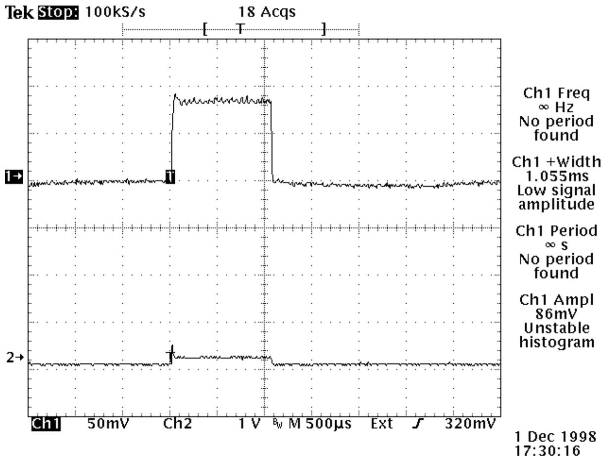
Figure 3.3: 43-mA ion-beam pulse (upper signal, 25 mA/div) from the R&D Ion Source at 12% duty factor. The discharge was cesium enhanced, but the source was not equipped with an electron-separating magnetic field or a dumping electrode. The electrons in the extracted beam were separated from the ions inside the Faraday cup and reached a current of 90 mA (lower signal, 500 mA/div).
