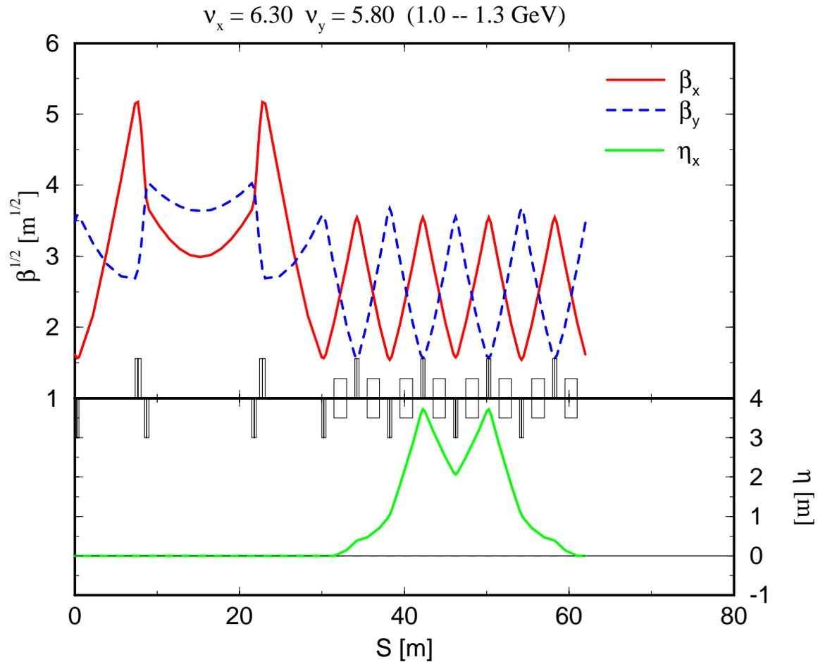
Figure 3.10: An alternative SNS Ring hybrid lattice with FODO arc and doublet straight sections.
