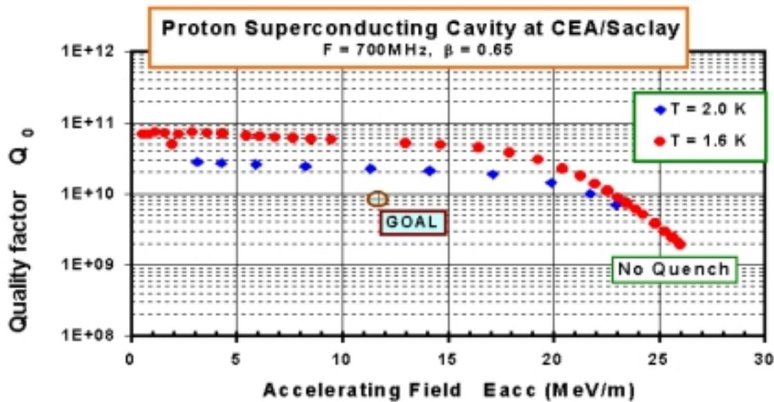
Figure 3.33:  $Q_0$  vs.  $E_{acc}$  plot for a single-cell niobium cavity for proton. (Note that the obtained performance by far exceeds the design goal)
