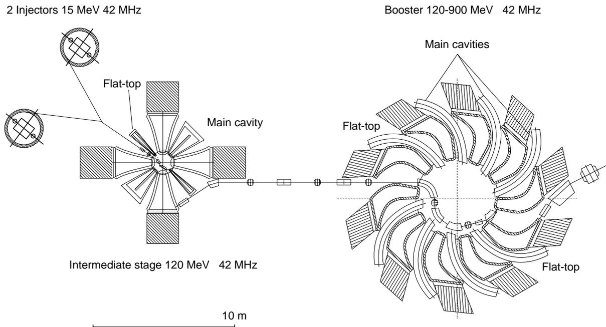
Figure 3.22: The full cyclotron high intensity accelerator layout proposed to drive a  $k = 0.98$  EA [1].
