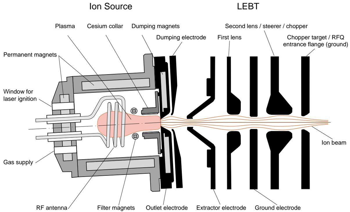
Figure 3.2: Schematic of Startup Ion-Source and Startup LEBT. Note that the actual filter and electron-dumping magnetic fields are oriented orthogonally to the illustration plane. The size of the ion beam is greatly exaggerated in this schematic to emphasize the focusing action of the double-lens system.
