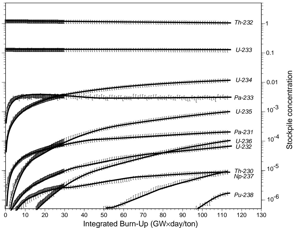
Figure 3.25: Evolution as a function of burnup of the stockpile of the main elements present in the EA fuel [1].
