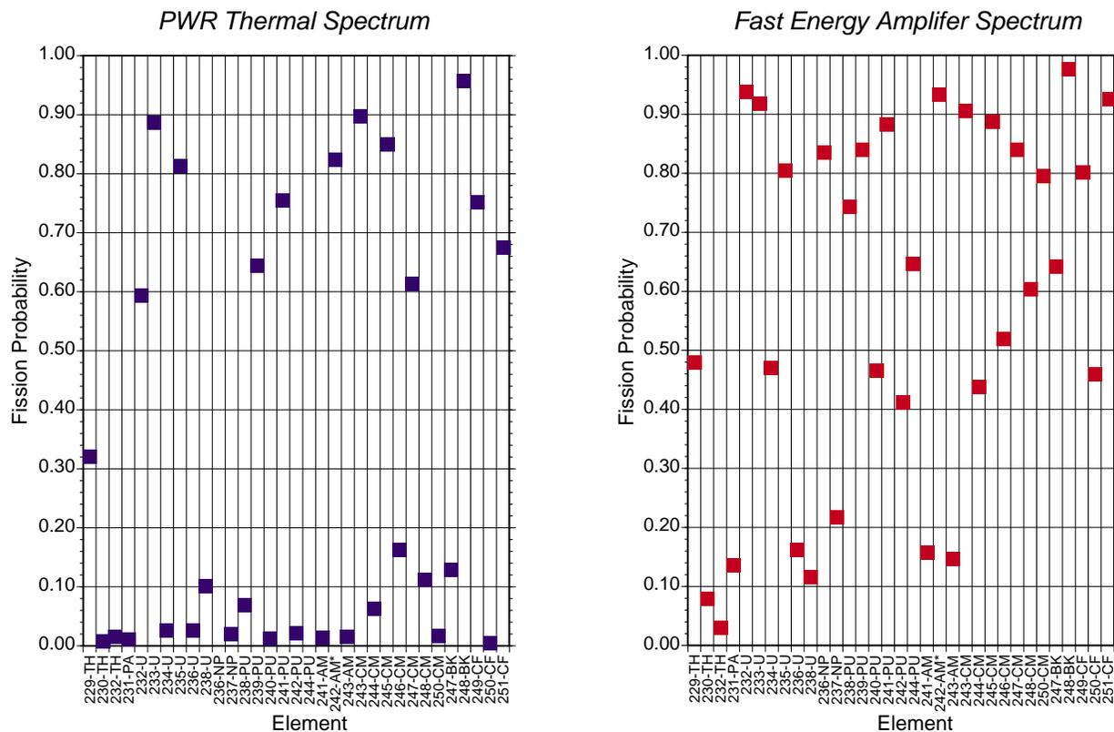
Figure 3.20: Comparison of fission and capture probabilities of actinides for thermal and fast neutron fluxes.
