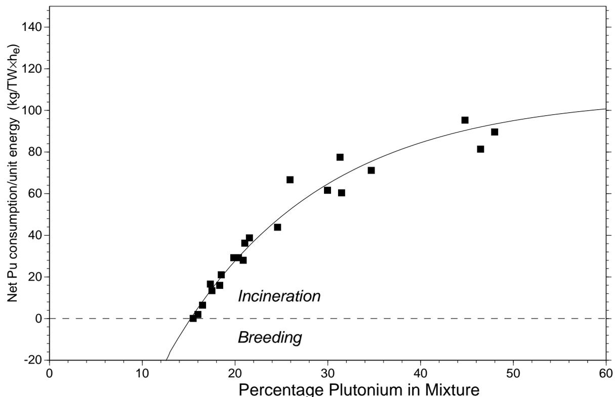
Figure 3.24: Net plutonium consumption per unit energy in a uranium-plutonium fast breeder (CAPRA [7]) as a function of plutonium concentration. Note that the unit is kg/TW×h electric and not thermal.
