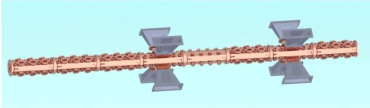
Figure 3.30: Computer view of the IPHI RFQ cavity (8 x 1m long)
