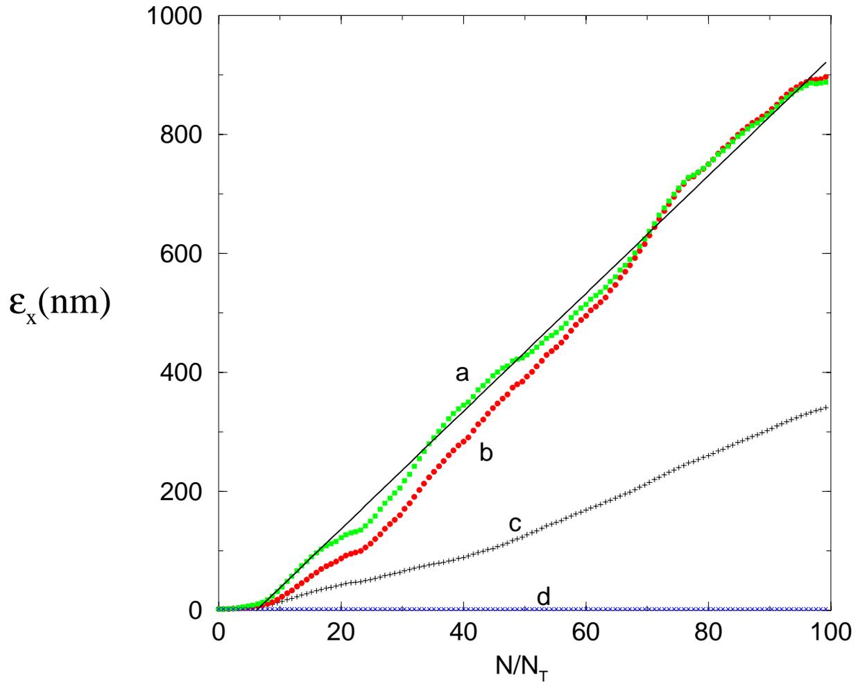
Figure 5.8: Emittance versus the fraction of total stages traversed at 2.5 TeV, with jitters  $\sigma_D = 1\mu$ .
