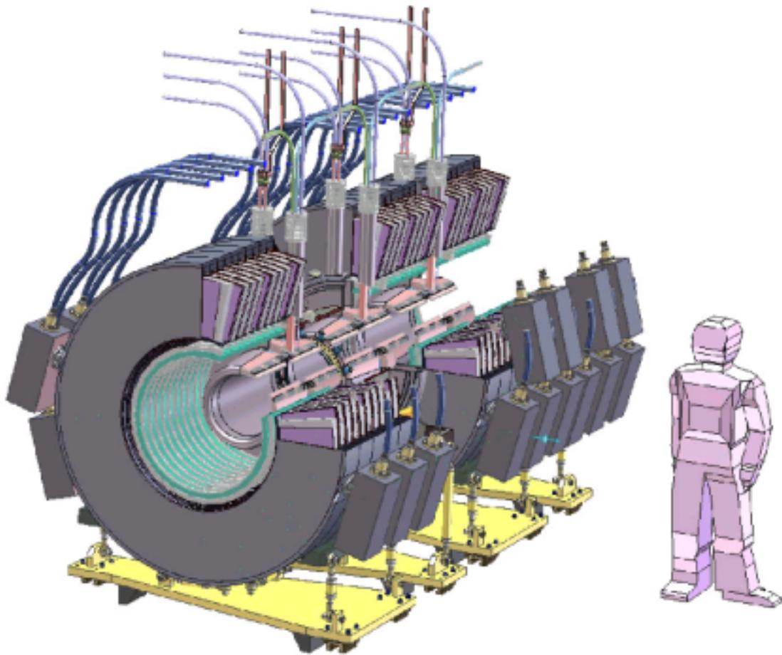
Figure 3.14: Sketch of an induction cell with integrated sc 3 T coils.
