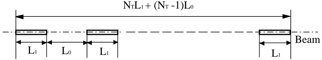
Figure 5.4: The layout of the aligned tubes in a laser-wakefield accelerator.
