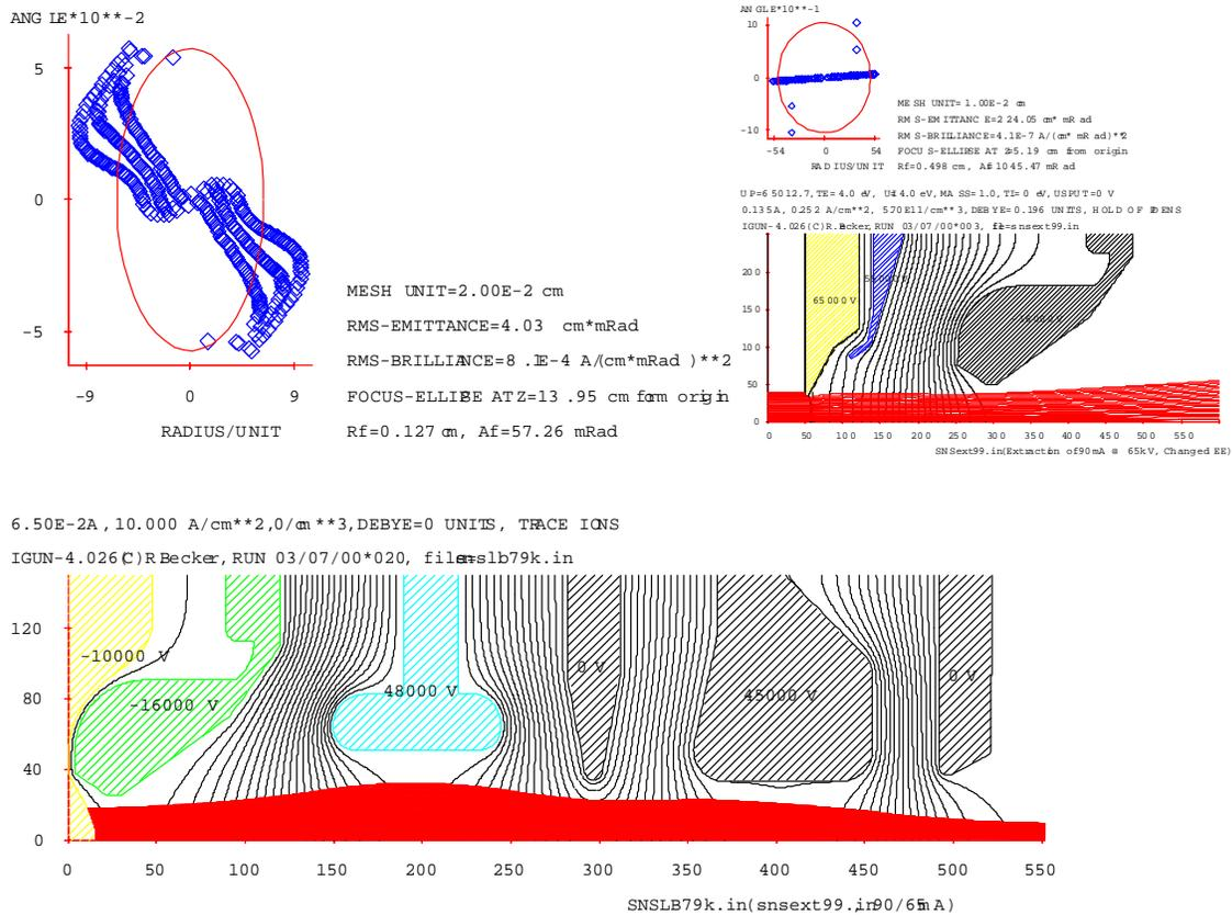
Figure 3.5: Production LEBT with beam trajectories simulated by IGUN. Assumed beam currents are 90 mA in the first part of the extraction gap and 65 mA elsewhere. The Twiss parameters in the exit plane are  $\alpha = 1.68$  and  $\beta = 0.090$  m, with a normalized rms emittance (converted to  $x/x'$  equivalent) of  $0.093 \pi$  mm mrad.
