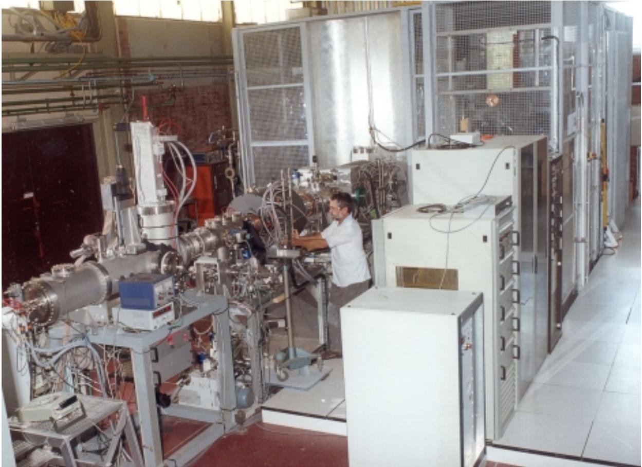
Figure 3.29: The high-intensity ECR source SILHI, LEBT and emittance measurement unit.
