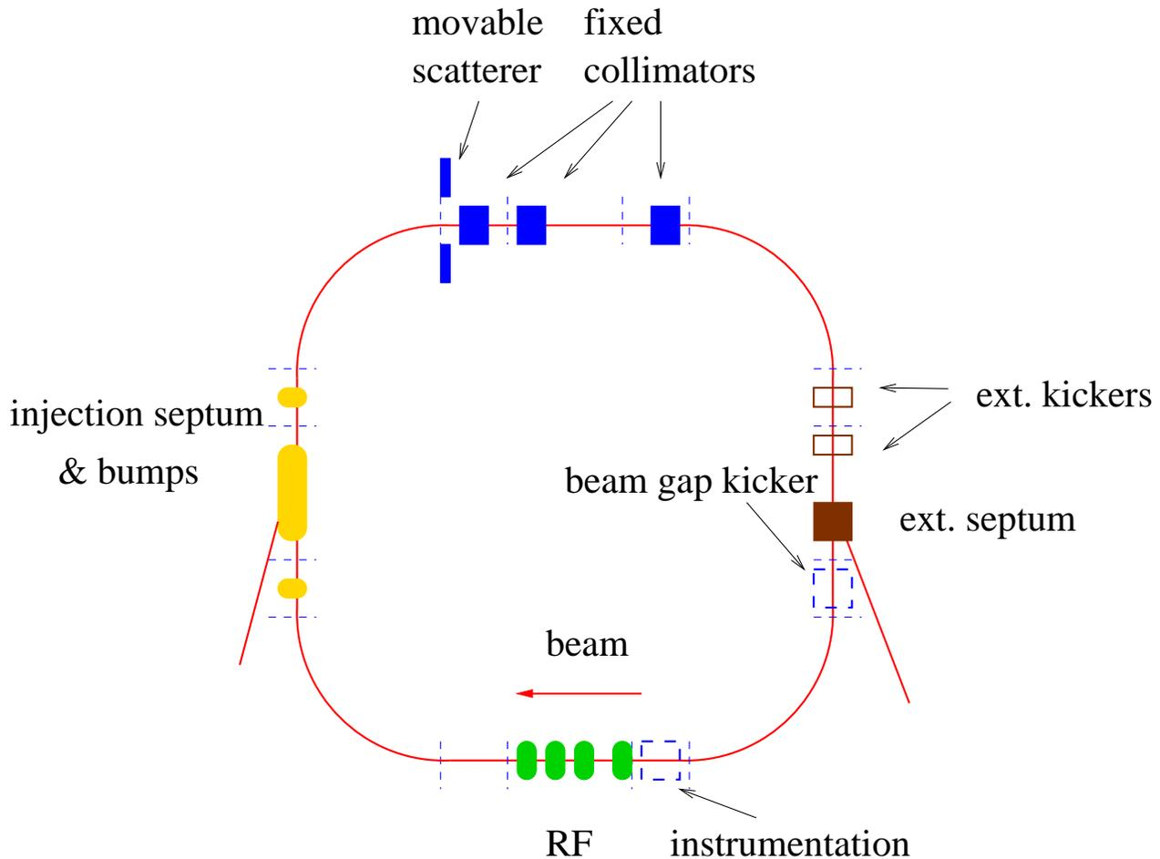
Figure 3.9: Schematic layout of the LINAC-accumulator ring indicating sections for injection, collimation, beam gap cleaning, RF system, instrumentation, and extraction.
