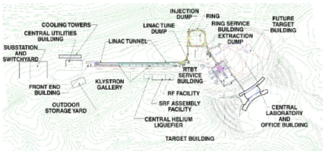
Figure 3.1: Schematic layout of the Spallation Neutron Source.
