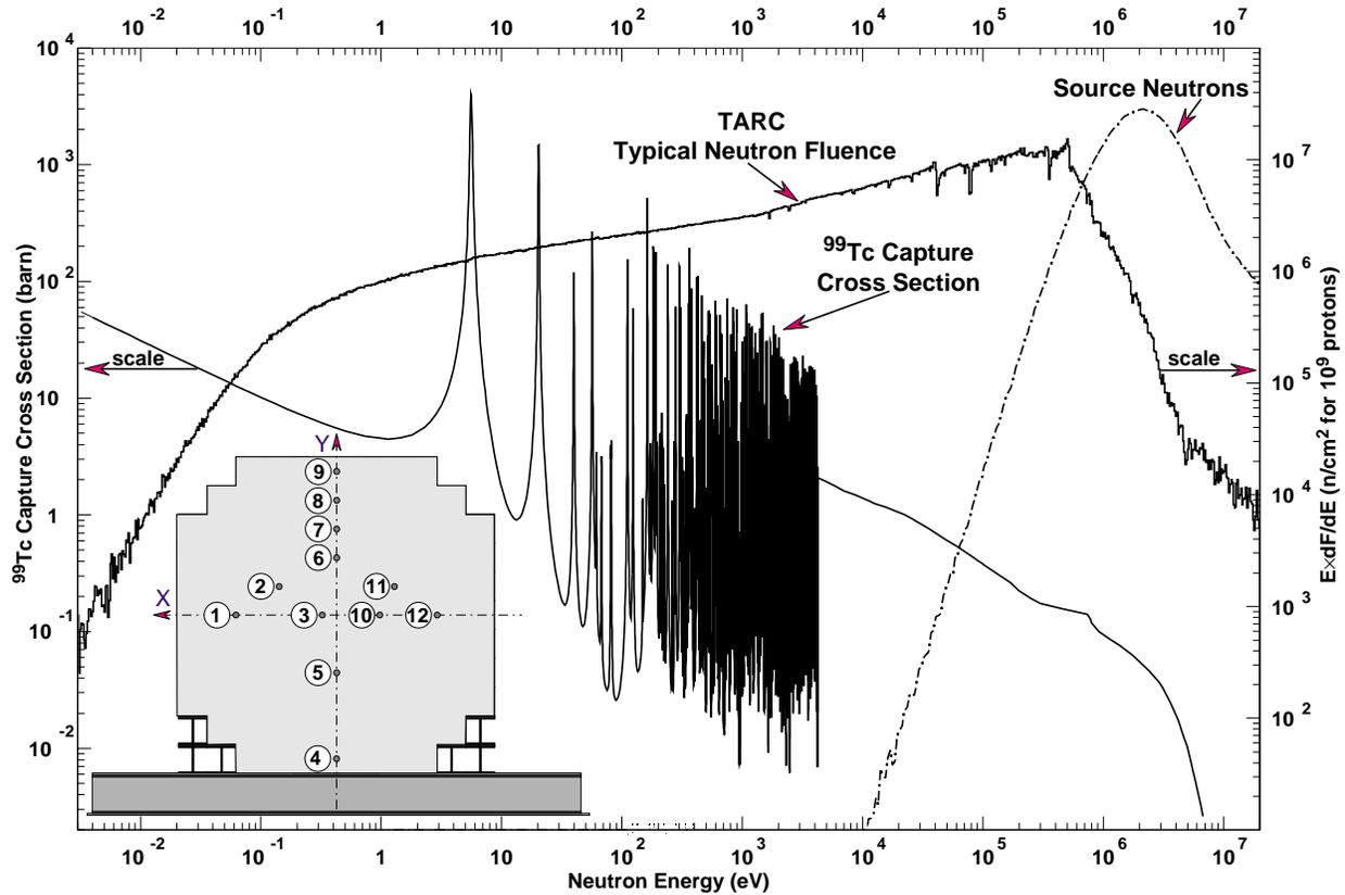
Figure 3.27: Illustration of the Adiabatic Resonance Crossing principle, showing how the presence of lead transforms the spallation neutron energy distribution into a flat flux distribution of slowing down neutrons, with iso-lethargic steps smaller than the width of cross-section resonances where they will be captured with high probability. A sketch of the 334 ton TARC lead volume is also shown.
