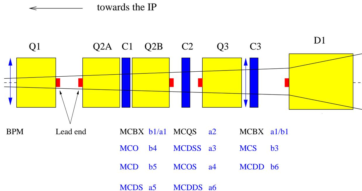
Figure 4.1: Schematic layout of the proposed LHC inner triplet region correction packages.
