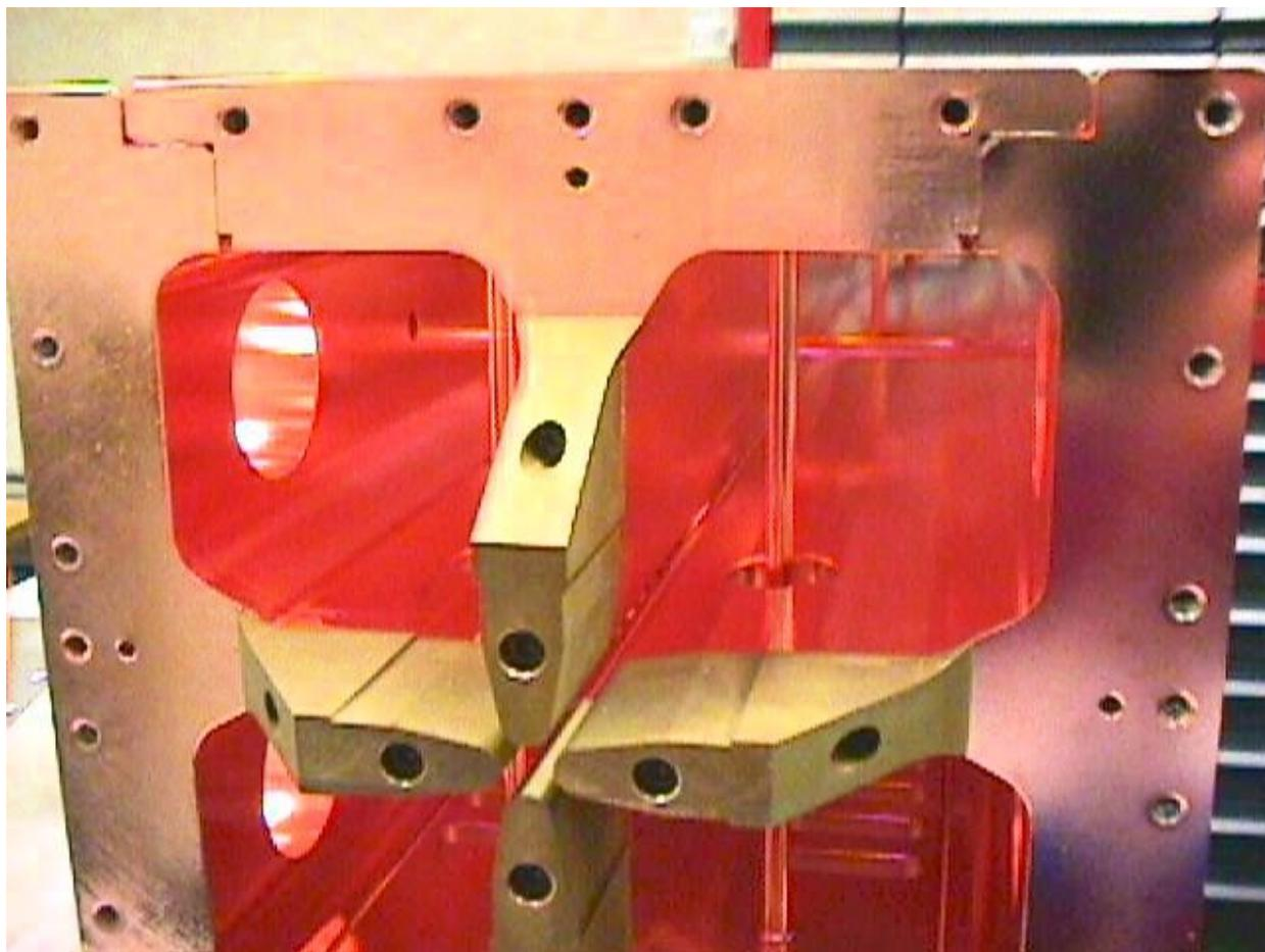
Figure 3.7: Pi-mode stabilizer rods within RFQ structure
