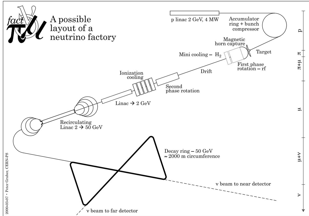
Figure 3.11: Possible layout of an European Neutrino Factory.
