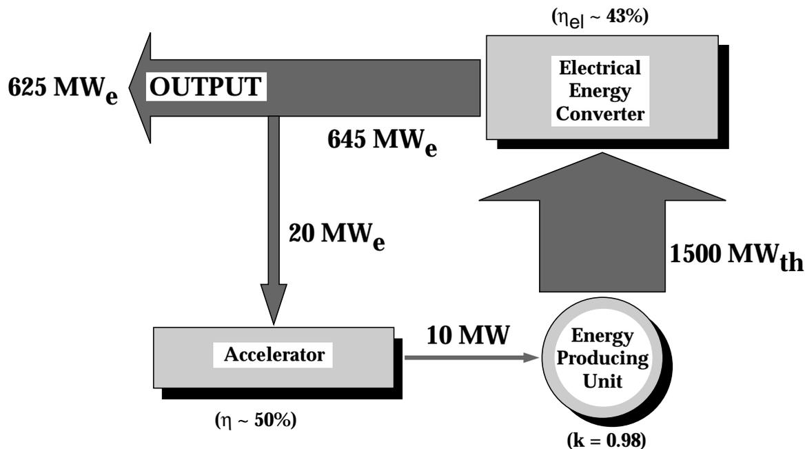
Figure 3.23: The energy amplification scheme in the standard EA system as proposed in Ref. [1].
