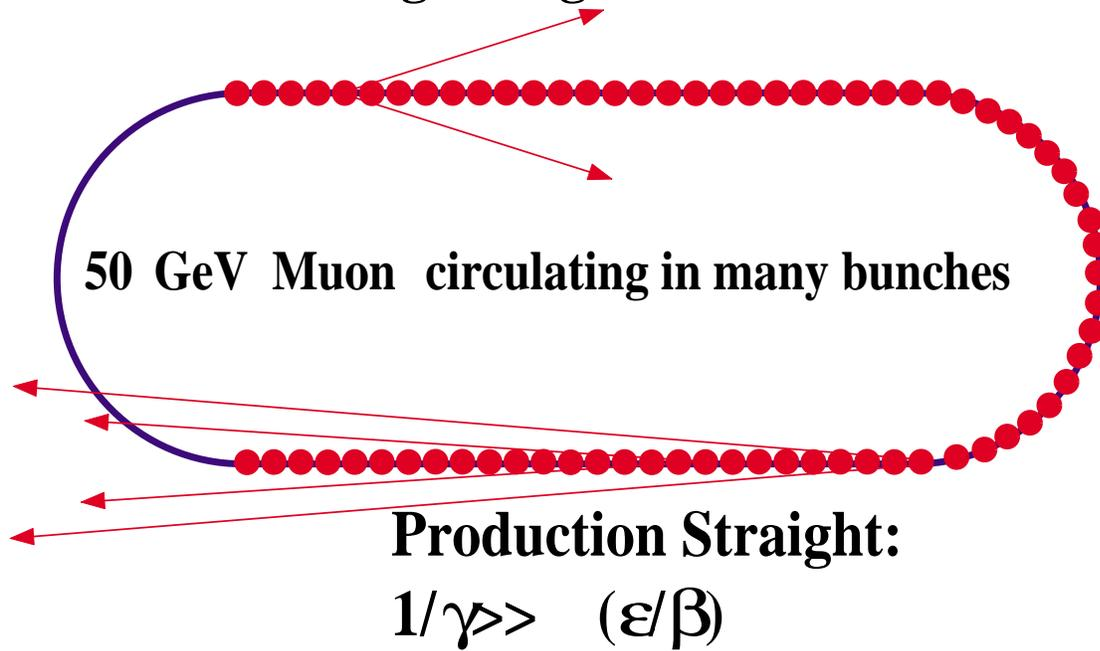
Figure 3.12: Sketch of a Muon storage ring with two long straight sections.
