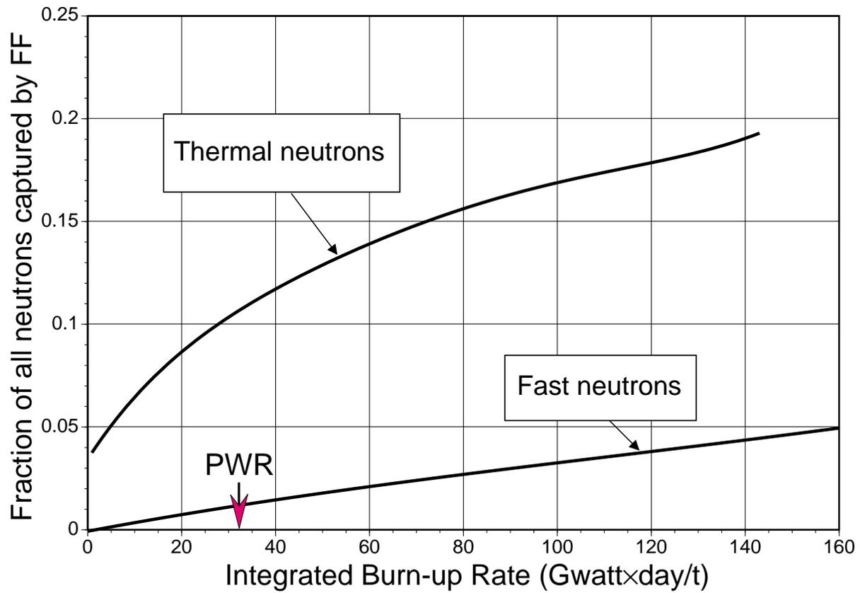
Figure 3.21: Fraction of neutron captures on fission fragments (FF) for thermal and fast neutron fluxes, as a function of burnup. The maximum burnup for a PWR is indicated. For the EA the burnup is expected to reach 150 Gwatt×day/ton.
