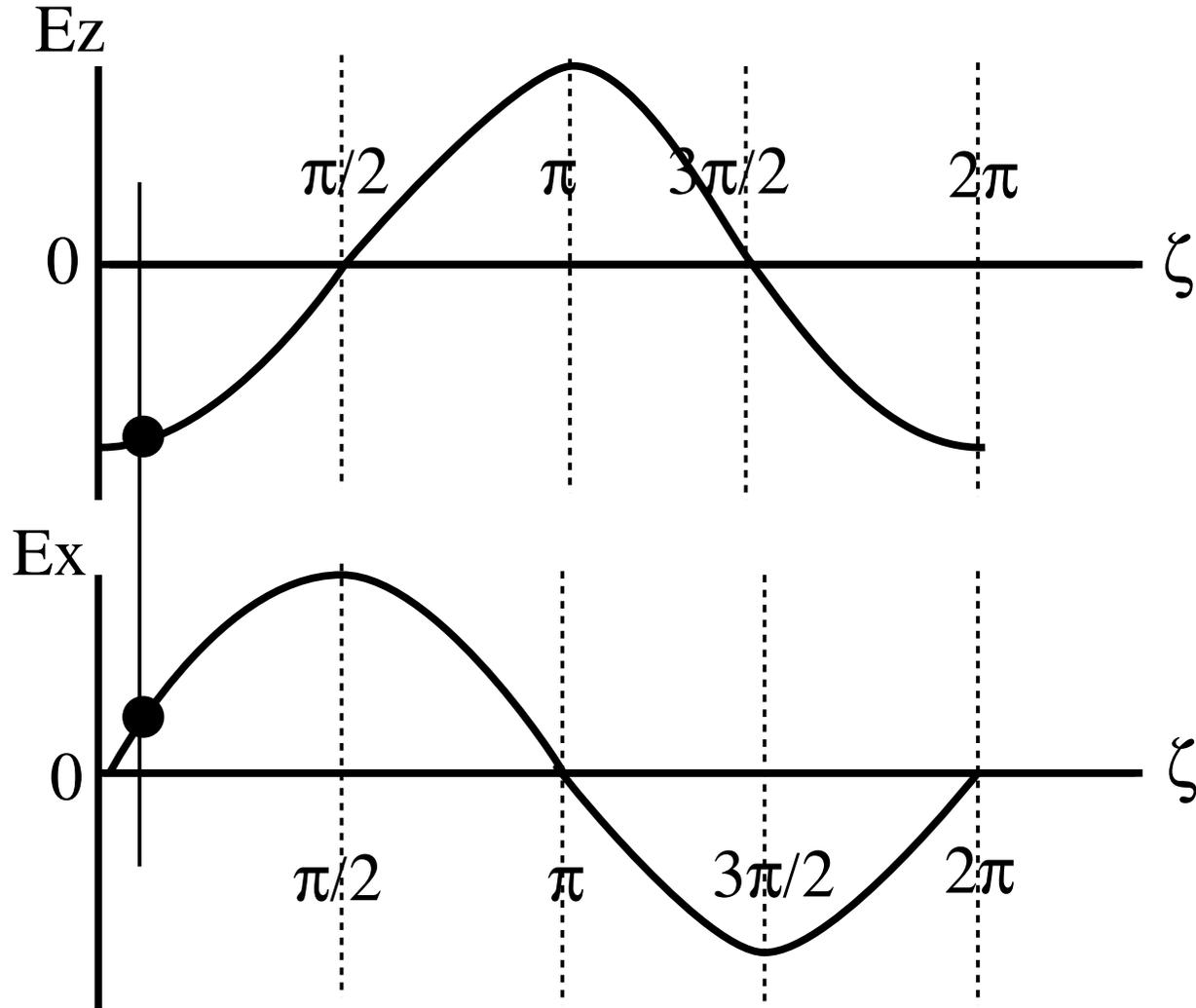
Figure 5.3: Sinusoidal oscillations of the longitudinal and the transverse components of wakefield as a function of the phase angle  $\zeta$ .
