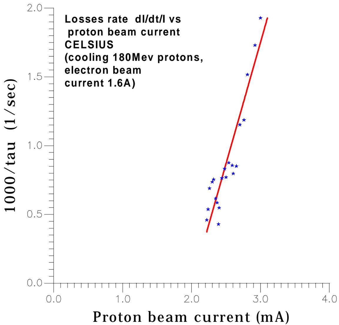
Figure 5.1: The losses of proton beam vs. proton beam current.
