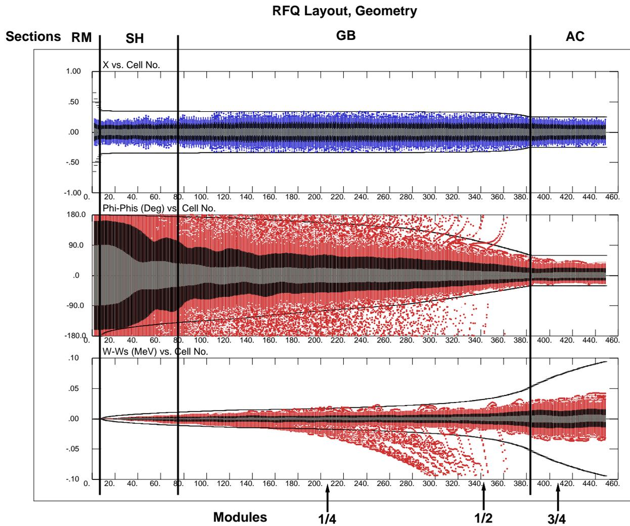
Figure 3.6: Transverse and longitudinal bunch widths, RFQ and module sections
