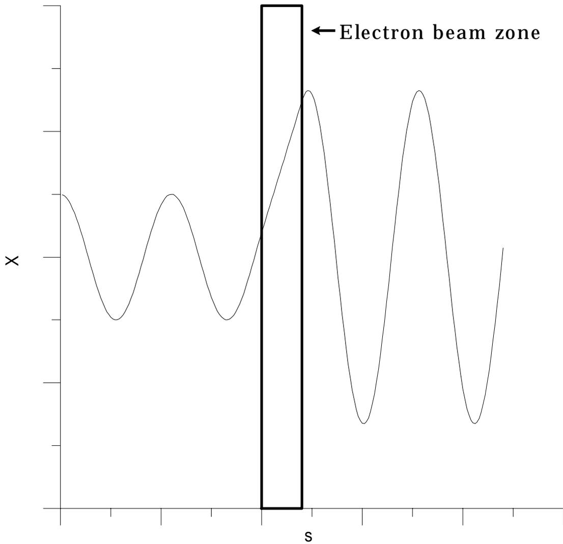
Figure 5.2: Simplified model of “electron heating”. The beam travels from the left to the right in the figure. A cloud of ions performs transverse or longitudinal plasma oscillations. Inside the electron beam, the restoring force disappears because the electrical fields are neutralized by the electrons, thus the ion cloud drifts to a larger plasma oscillation amplitude.
