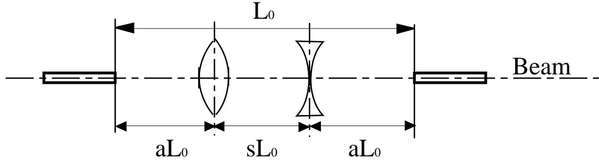
Figure 5.5: The layout of a quadrupole doublet within a gap.
