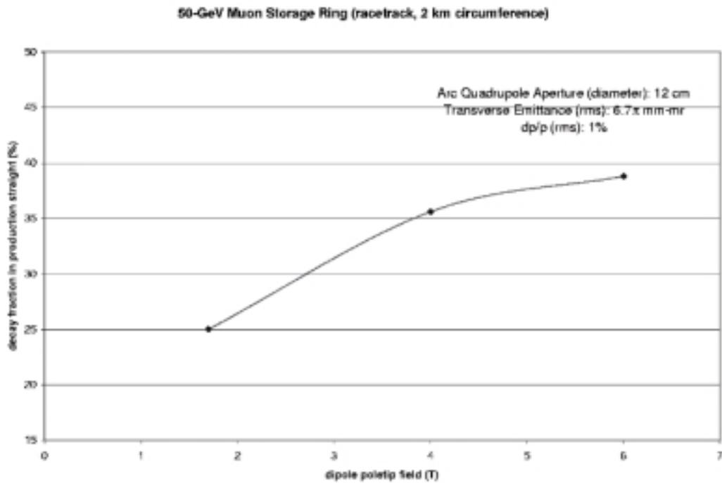
Figure 3.16: Muon yield versus bend strength assuming the maximum depth to be used for the storage ring tunnel at angle of  $13^\circ$ .
