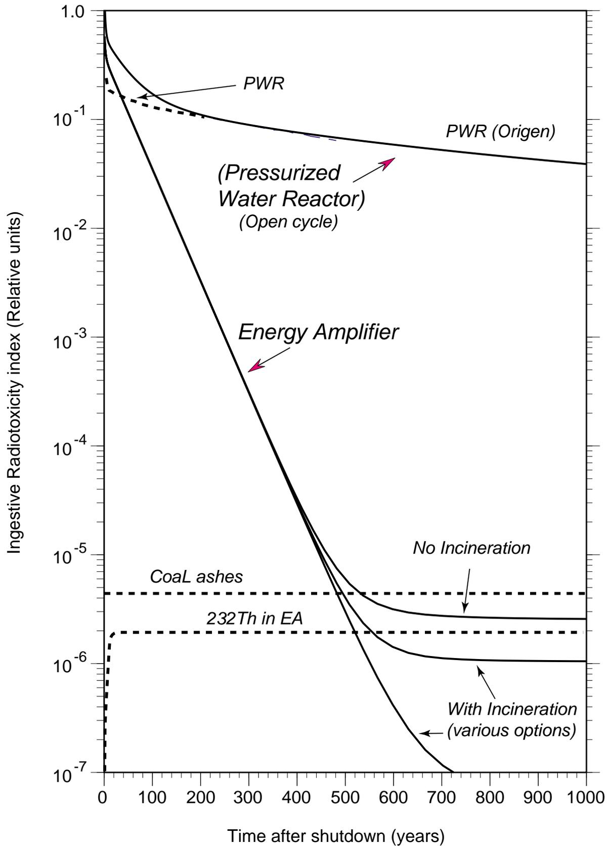
Figure 3.26: Evolution of the potential radiotoxicity of nuclear waste for PWR, EA and coal burning power station, showing that in the EA, the long-term radiotoxicity can be 4 orders of magnitude smaller than in a PWR in open cycle and is dominated by LLFF if no further incineration is performed (adapted from Ref. [11]).
