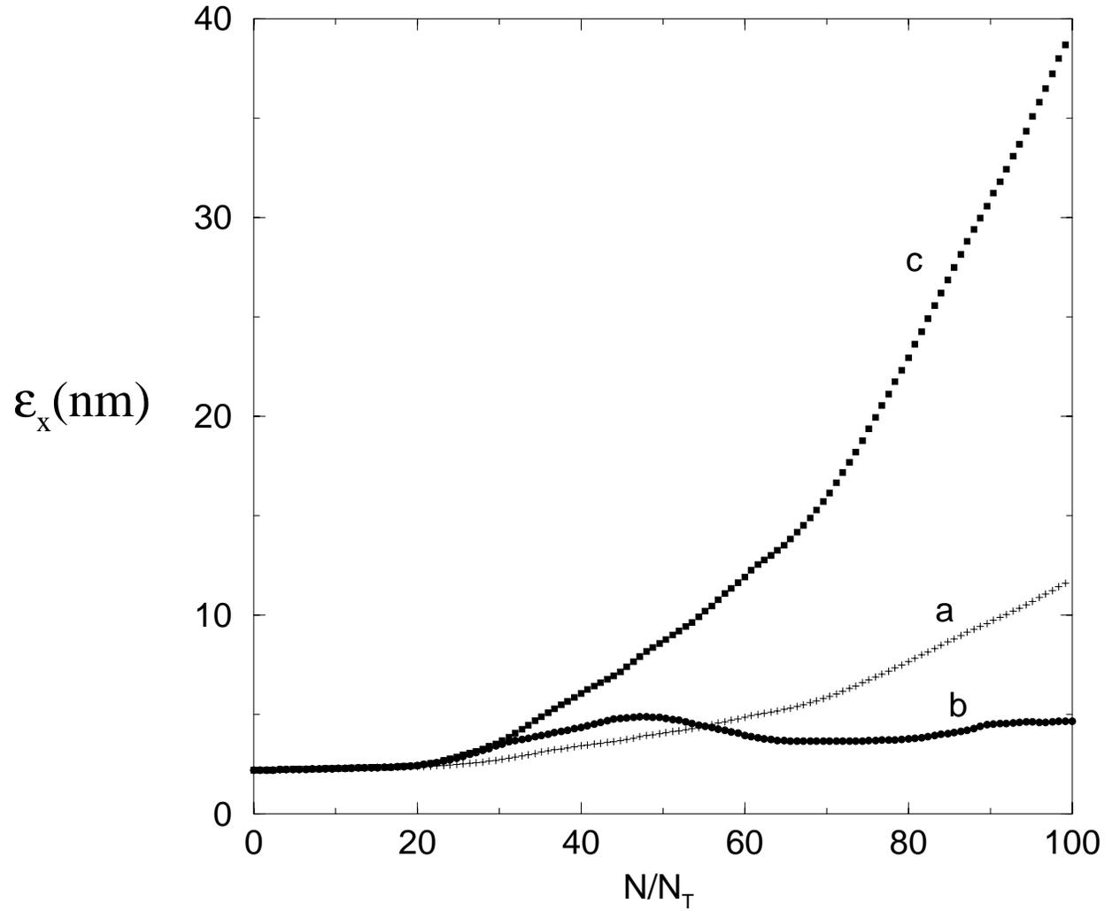
Figure 5.10: Emittance versus the percentage of total stages traversed at 2.5 TeV for an accelerator with a total of 500 superunits, where there are 100 stages per superunit.
