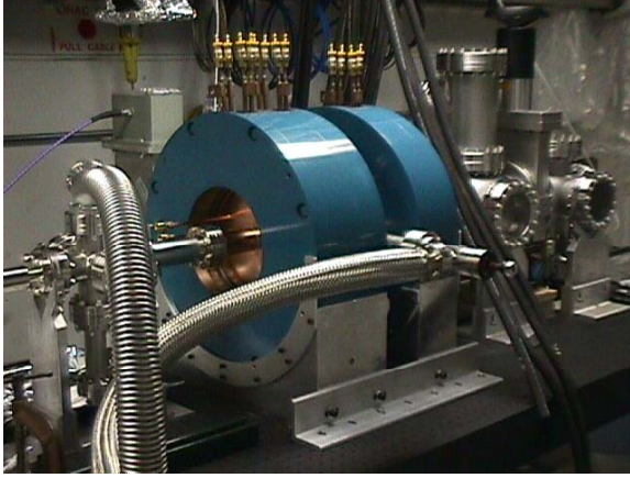
Figure 2. The new RF photocathode gun installed at the AWA during recent commissioning.
