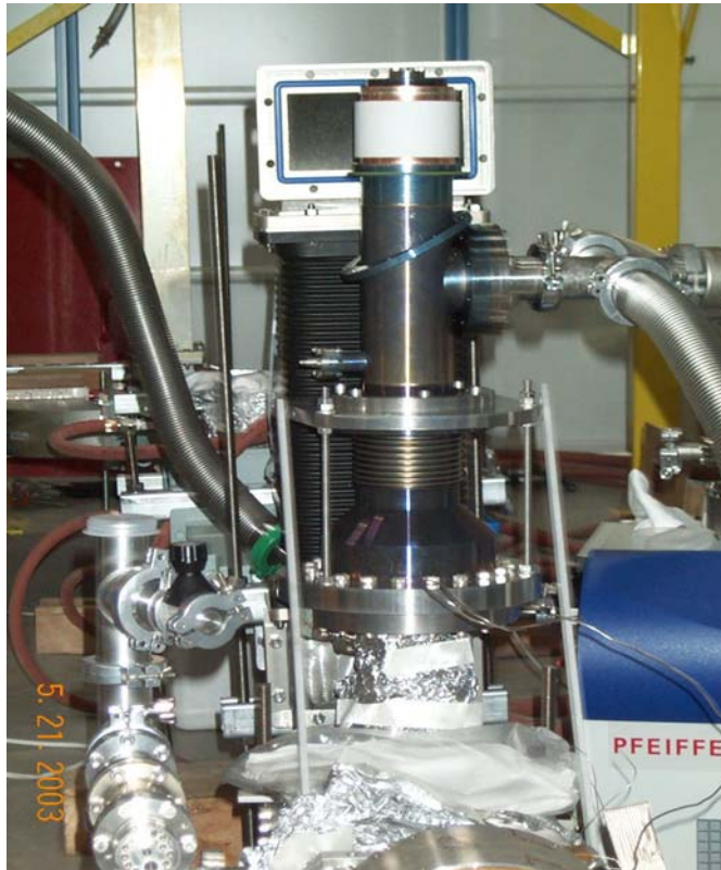
Figure 1. Power Coupler mounted on the wave-guide test bench. The ceramic window which separates the coupler vacuum from the wave-guide is visible at the top of the coupler.
