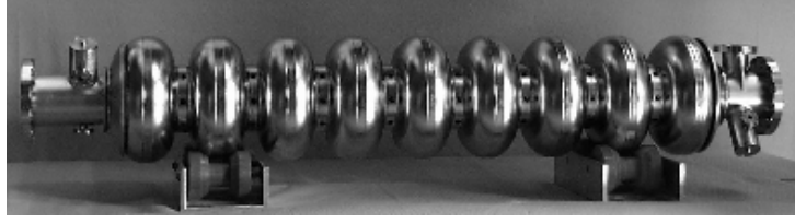
Figure 2: Superconducting 1.3 GHz 9-cell cavity for the TESLA Test Facility.
