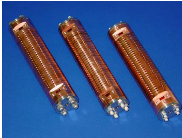
Figure 1: Copper, tungsten iris and molybdenum iris 30 GHz accelerating structures.
