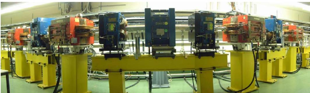
**Figure 6:** The bunch length manipulation chicane.
