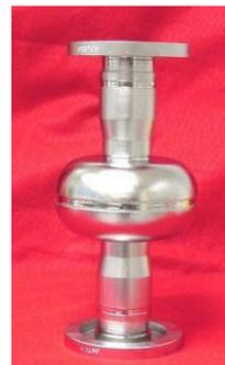
**Figure 2.14:** Cutting-edge SCRF R&D. top-left: ICHIRO single-cells being prepared for testing at KEK. Top right: world-record performance from novel shape single-cells (ICHIRO and Cornell's reentrant cavity). Bottom left: large-grain niobium disk (JLAB). Bottom-right: single-cell cavity produced from large-grain niobium material (JLAB).
