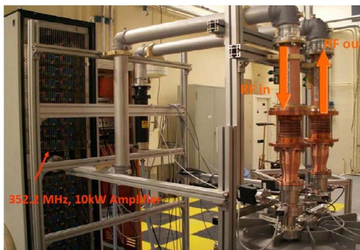
**Figure 7:** RF conditioning of the Spoke power couplers.
