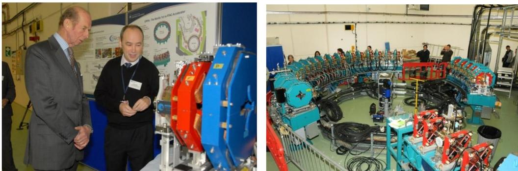
**Figure 2:** An EMMA cell with a royal visitor (left) and 4 EMMA girders in place (right), with the end of the injection line at the bottom right of the photograph.
