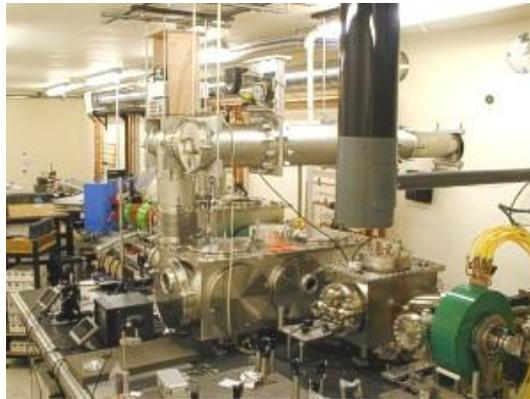
**Figure 1:** The ALPHA-X beam-line and plasma wakefield accelerator.
