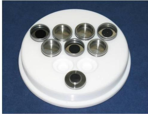
Figure 5: GaAs photocathodes on molybdenum substrate
