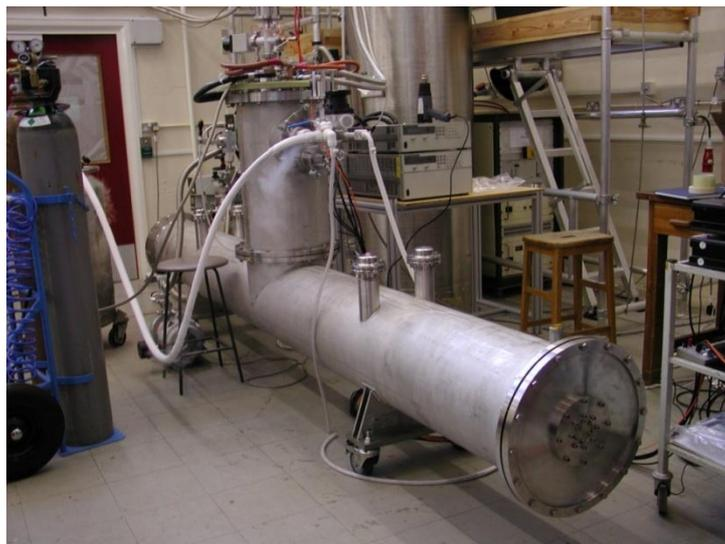
**Figure 1.** The 4m long cryomodule under commissioning at RAL.
