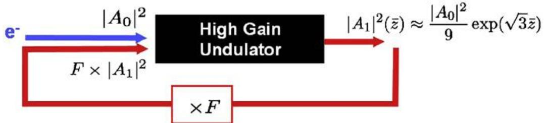
**Figure 2:** Schematic showing a generic high gain RAFEL system.
