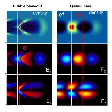
**Figure** Wakes 3: generated in the bubble (left column) and quasi-linear (right column) regimes by a laser pulse with  $a_0=4$  (*left*) and  $a_0=1$ (right).Top figures are axial electric field, central figures are density, and bottom figures are transverse electric fields. The black boxes indicate the accelerating/focusing regions for electrons, and the green boxes are for positrons (Courtesy of C. Benedetti et al., LBNL).
