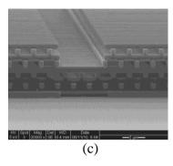
**Figure 1:** Recently constructed prototypes of (a) the 1D dual grating accelerator structure with 800 nm period. (Stanford University), (b) The 2D photonic capillary wafer accelerator structure with transverse size about 700 microns (Income Inc.). (c) 9-layer half structure of the 3D photonic woodpile with rectangular defect region where the particle beam traverses into the page (Stanford University).
