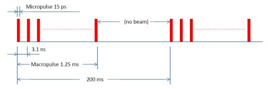
**Figure 9:** H<sup>-</sup> pulse structure of Project X.
