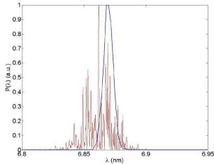
**Figure 11:** Typical wavelength spectral distribution of a single SASE FEL pulse. Red: calculated for a typical SASE process starting from shot noise. Blue: with external seeding.
