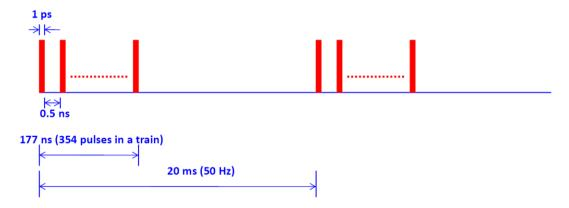
**Figure 6:** CLIC-based γγ collider beam structure.
