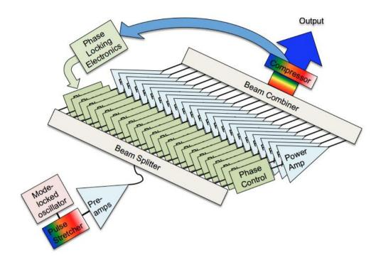
**Figure 13:** Conceptual outline of a coherently combined fiber laser array.
