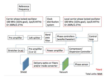
**Figure 3:** The laser system baseline design is shown. The red outlined boxes highlight the challenging portions of the system. A total of M local oscillators will be built and split N times, giving a total of M×N laser coupled accelerator structures.
