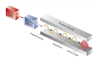
**Figure 1:** Laser-plasma acceleration: An intense laser pulse drives a plasma wave (wake) in a plasma channel, which also guides the laser pulse and prevents diffraction. Plasma background electrons injected with the proper phase can be accelerated and focused by the wake [1].
