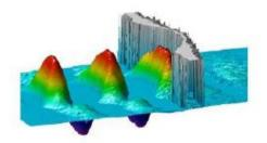
**Figure 7:** The process of RPA acceleration. The laser is impinging on the ultra-thin foil, building up a compressed layer of electrons, which in return transfers momentum to all the particles in the foil. [39-40]
