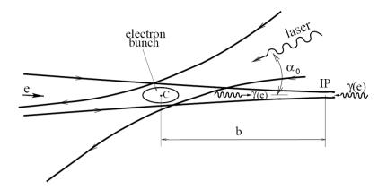
**Figure 5:** Illustration of the principle of a  $\gamma\gamma$  collider.
