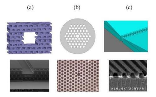
**Figure 4:** Three dielectric laser accelerator topologies: (a) a 3D silicon photonic crystal structure, (b) a hollow-core photonic bandgap fiber, and (c) a dual-grating structure, showing conceptual illustration (top) and recently fabricated structures (bottom).
