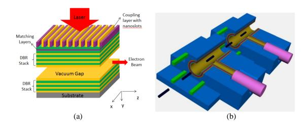
**Figure 2:** Proposed structures that are in development: (a) The 1D MAP Bragg reflector accelerator structure (UCLA) and (b) The 1D Omniguide dielectric accelerator. The particle beam traverses the cylindrical accelerator cavities on a path indicated by the dashed line (Purdue University).
