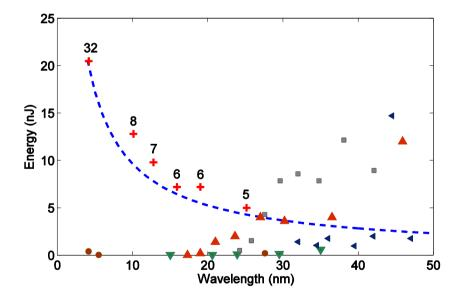
**Figure 12:** HHG state-of-the art, with the blue dashed line indicating 100 times the shot noise at that wavelength. The number by the crosses indicate the number of QPM jets needed. The triangles refer to HHG in Ar and Xe and the circles to QPM in capillaries. The squares are achieved with two-colour mixing.
