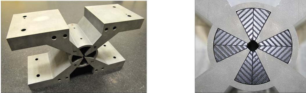
**Figure 6:** The prototype core elements: the monolithic Permendur structure (left) and a details of the PM wedges inserted in the central part (right). The lines on the PM surface indicate the magnetization directions.
