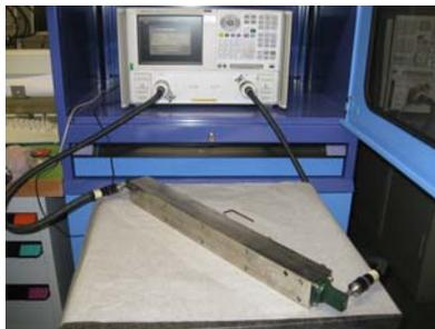
**Figure 5:** Measurements setup: network analyzer, the transmission coefficient  $S_{21}$  of an X-band waveguide is measured.
