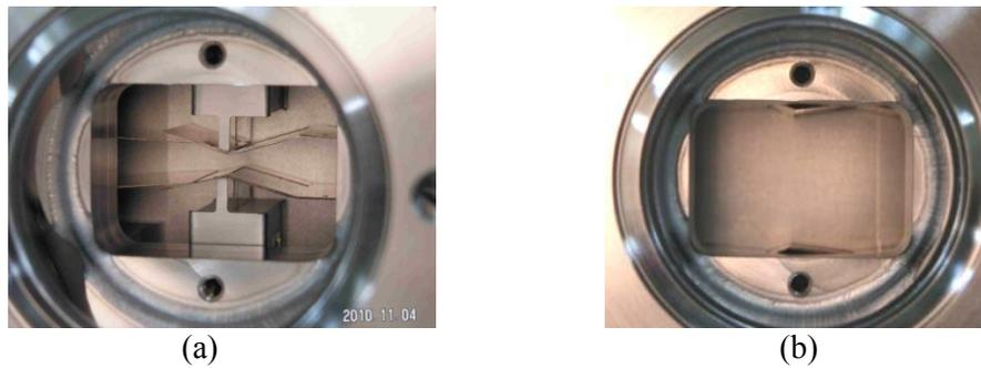
**Figure 11:** Photograph of the RF fingers with Al windows in (a) active mode and (b) shelter mode. The beam direction is from right to left.
